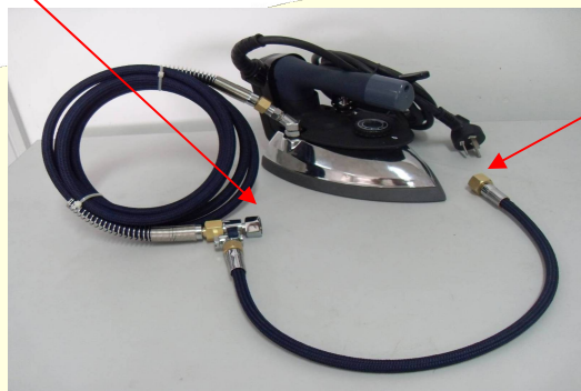
Steam Drain Line
